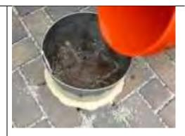
Infiltration test using ASTM C-1781
